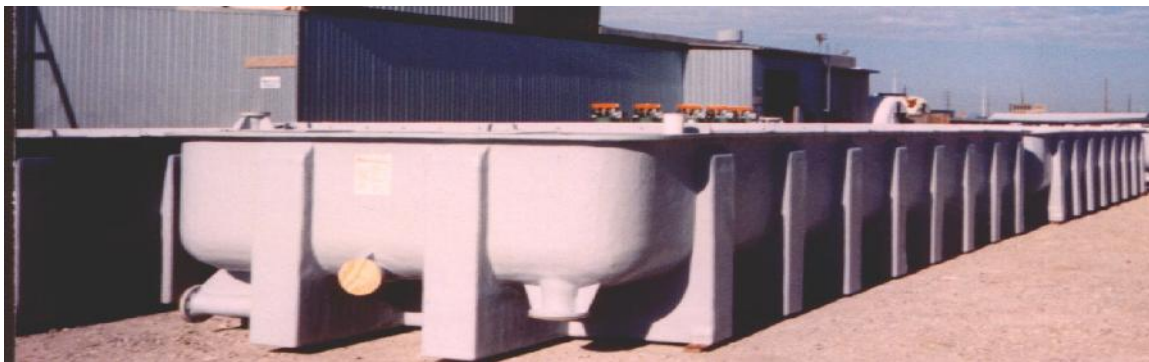
QPEC 9' x 34' Solvent Extraction System
