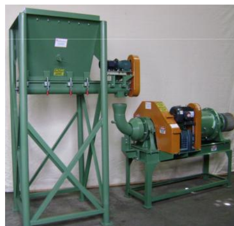
QPEC 16" x 48" Ball Mill and Hopper Screw Conveyor
