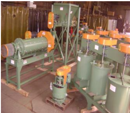
QPEC Equipment 16" x 48" Ball Mill, Hopper Screw Conveyor, Agitators, Flot Cells, & Pump
