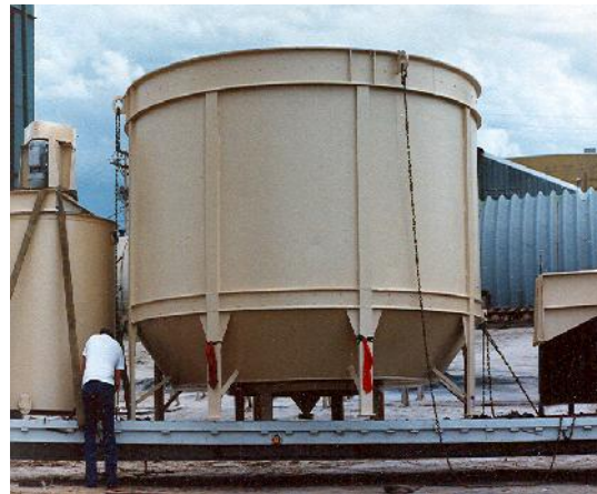
Rebuilt 16' X 12' Dia. Thickener Tank with Superstructure and 8'x8' Agitator Tanks
