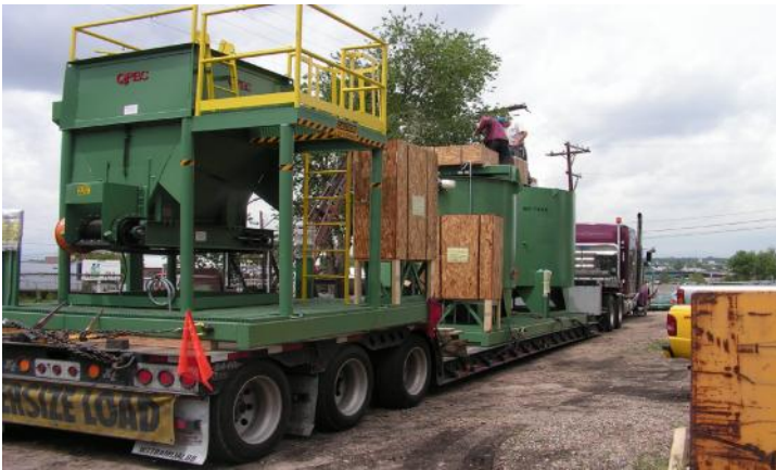
QPEC skid mounted Hopper Belt Feeder in transit with 2 QPEC skid Mounted Thickner Tanks to Australia
