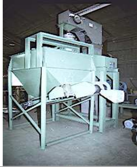
QPEC Grinding Module Ball Mill with Hopper
