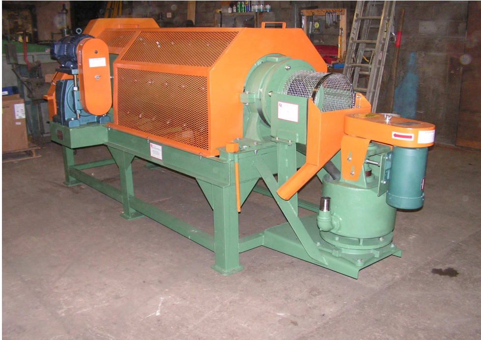
24" Ball-Rod Mill x 64" with safety cage and 1" vertical sand pump
