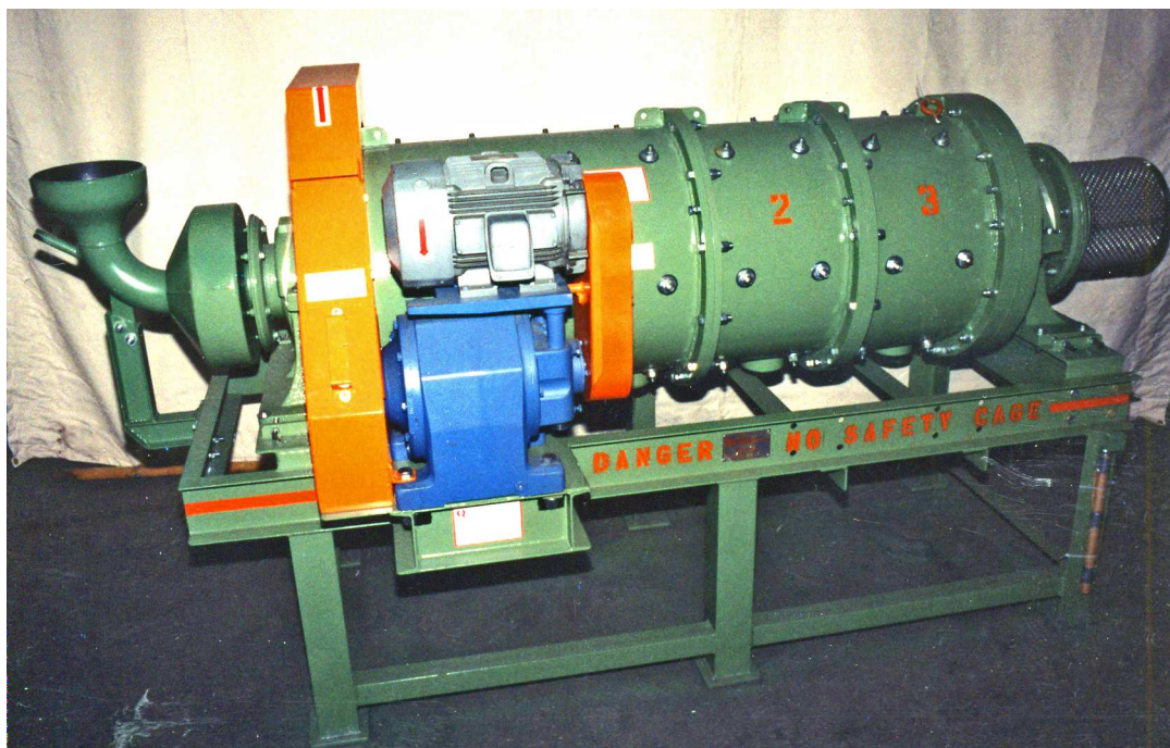
16" Ball-Rod Mill 3-sectional x 32", x 48", x 64"
